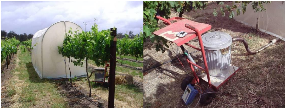
Figure 1. Field smoke application apparatus showing smoke tent with vines enclosed (left) and smoke generator (right).
