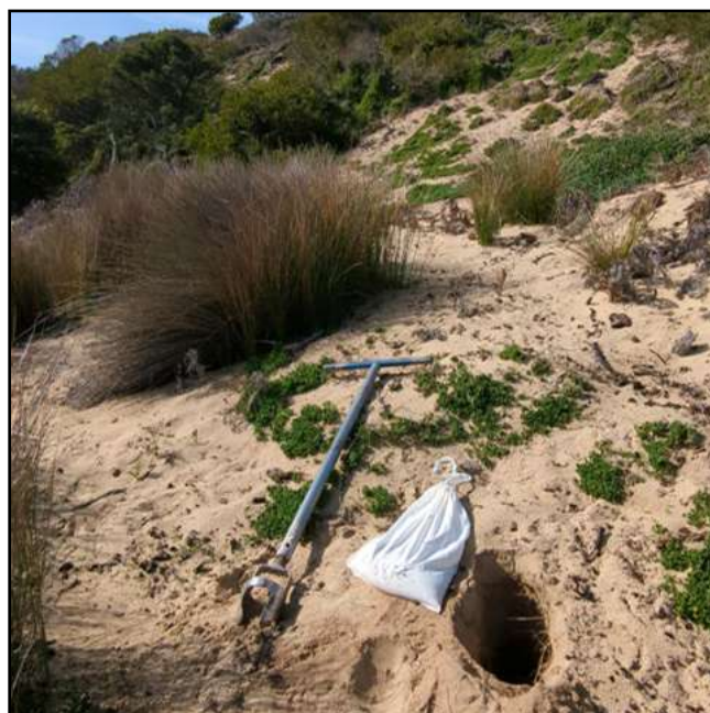
Figure 20. Handheld auger used for sampling sand at depths up to 1 m.
