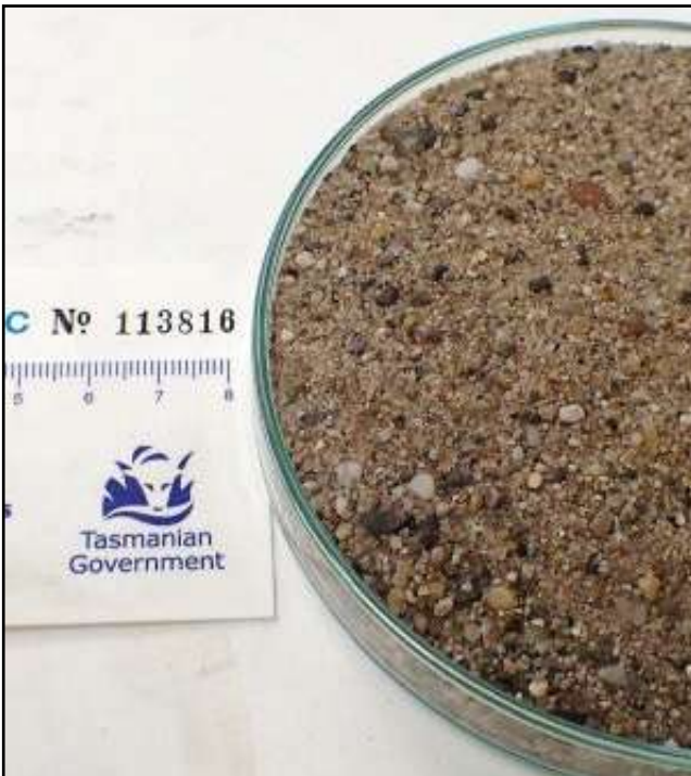
Figure 7. The Goats Bluff washed coarse sand is the only sand product mined in SE Tasmania that meets specifications for fine aggregate grade envelope for concrete production.
